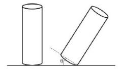
In a simple experiment, the stability of the bottle filled with different amount of shampoo volume is observed. The bottle is tilted from one side and then released. Let the angle  $\Theta$  depicts the critical angular displacement resulting in the bottle losing its stability and tipping over. Choose the graph correctly depicting the fraction f of shampoo filled (f = 1 corresponds to completely filled) vs the tipping angle  $\Theta$ .
