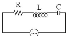
To maximize the average power supply, current should be maximum.
